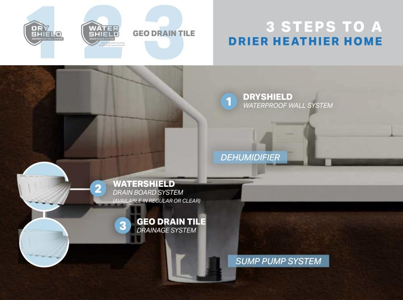
DRYSHIELD WATERPROOF WALL SYSTEM WATERSHIELD DRAIN BOARD SYSTEM **GEO DRAIN TILE** DRAINAGE SYSTEM
