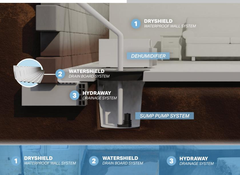
Directs basement water seepage below the slab to the interior drainage system. Stops the evaporative effect, helping to eliminate musty damp basement air.
